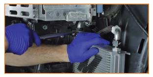
23. Install the shield bracket. Secure the top to the crash beam and the upper edge to the oil cooler. Torque the top bolt to the correct factory specifications.
