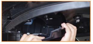
3. Disconnect the fog light on each side once you have access behind the splash shields. Depress the small tab at the end of the connector to separate the connection.
