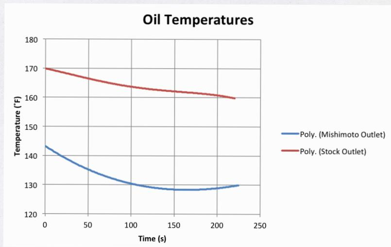
**Figure 7:** The Mishimoto oil cooler shows a 30° F lower outlet temperature compared to stock.
