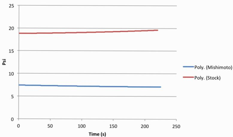
**Figure 9:** The Mishimoto oil cooler shows a dramatic 11 psi reduction in pressure loss.
