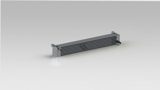
Figure 6: 3D CAD model of Mishimoto oil cooler
