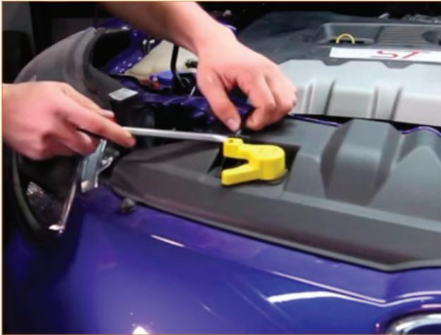
06. Remove the Torx screws and pop clips that secure the fender liner to the front bumper cover on both sides of the vehicle. There are two screws and one pop-clip on each side. (4x T30 Torx screws, 2x pop-clips)
