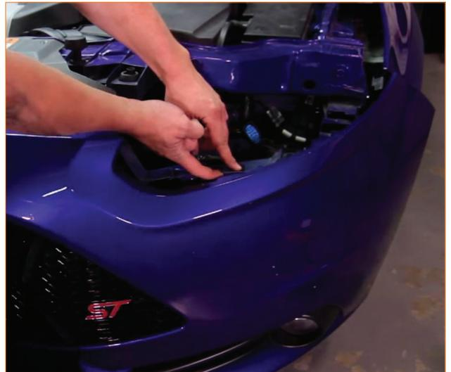
12. Remove the upper air shroud by releasing the two clips at the outside edges.
