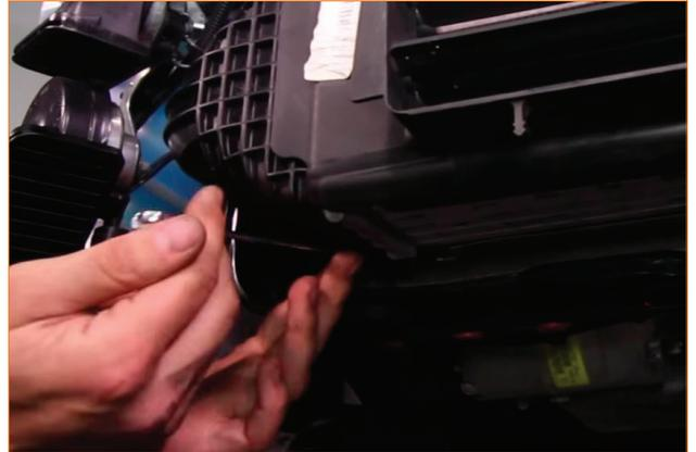
20. Remove the active grille shutters. The shutters are held in by four clips that secure it to the AC condenser. These can be released by hand. Then slide the active grille shutters down and remove them completely. They will not be reinstalled.
