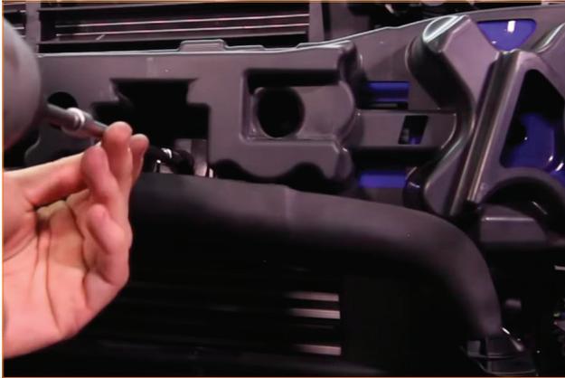
14. Disconnect the electrical connector for the active grille shutters. Release the two tree clips that secure the connector and harness to the vehicle. (2x tree-clips)
