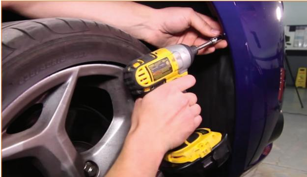
07. Remove the six pop-clips that secure the bottom of the front bumper cover to the front splash panel. (6x pop-clips)
