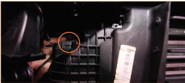
19. Remove the intercooler. Remove the two bolts that secure the intercooler. Then pull the intercooler forward and lower it to remove it completely. (2x 8mm bolts)
