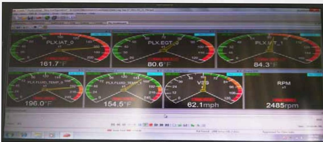
Fluid temperatures were taken from both the inlet and outlet of the 19-row oil cooler using a Mishimoto oil sandwich plate with PLX fluid temperature sensors. Oil pressure was also tested to ensure no dramatic pressure drop occurs when installing the large oil cooler.
