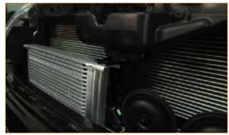
**7.** Using 10mm bolts, secure the oil cooler to the bracket. At this time be sure all mounting bracket bolts are tight.
