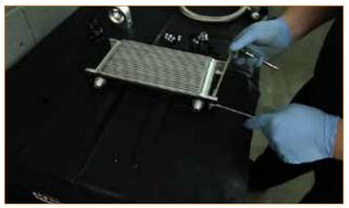
**2.** Line up the mounting bracket holes with the transmission cooler mounting points.
