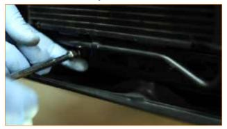
${\bf 5.}$  Next remove the third bolt located in the front bumper frame, as seen in the photo.
