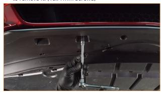
**04.** Remove the four screws that secure the rear splash panel to the vehicle. Then remove the splash panel from the vehicle. (4x 7mm screws)
