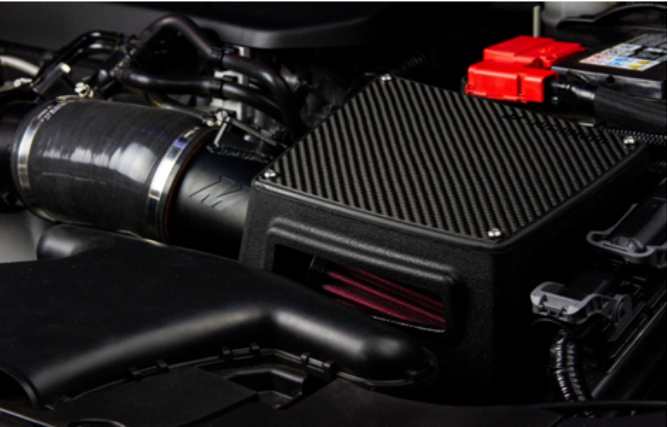
FIGURE 3: Mishimoto intake installed
