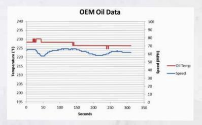
At cruising speeds, the OEM oil temperature is around 225-230 degrees F.
