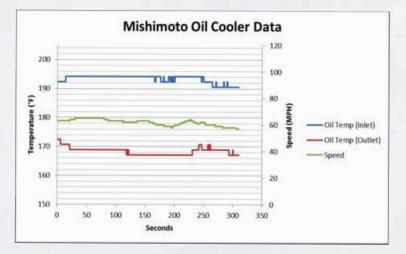
At cruising speeds, the oil temperatures entering the cooler are around 190-195 degrees F.
