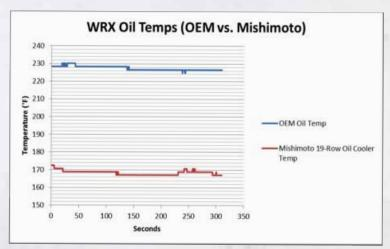
The graph above compares the temperatures of the oil returning to the engine with and without the oil cooler installed. A drop in temperature of roughly 60°F occurs when the WRX is equipped with the Mishimoto 19-row oil cooler.
