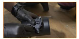
10. Transfer the grommets from the stock airbox to the Mishimoto airbox.
