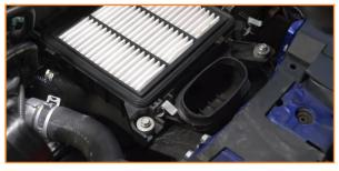
8. Remove the filter from the airbox. With the filter out, lift the airbox to disengage the peg at its base.
