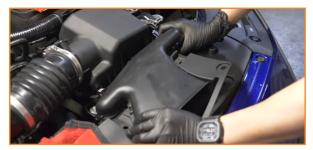
3. Before carrying out this next step, make sure the ignition is off, then you can disconnect the MAF sensor.
