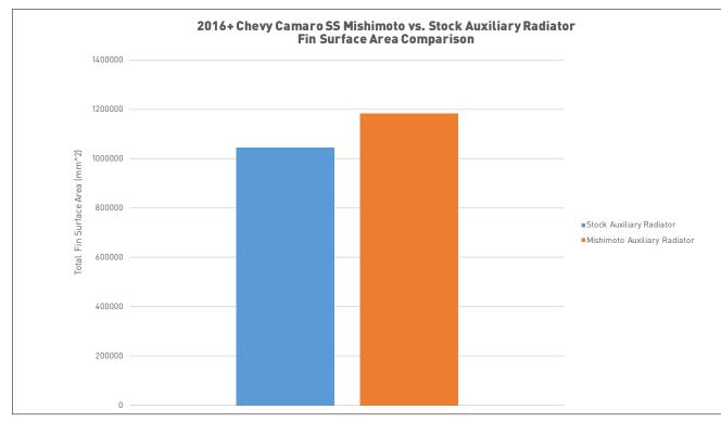
FIGURE 2: The Mishimoto auxiliary radiator features an increase in fin surface area, which promotes greater heat transfer.
