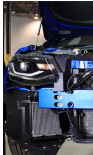
heat exchanger can be relatively tight, passing through as the core will still be the path of least resistance for airflow. While the design of the Camaro doesn't leave much room to increase the auxiliary radiator core sizes, the ducting allows for an increase in fin surface area, which will aid in increasing heat transfer. As shown in Figure 2,
