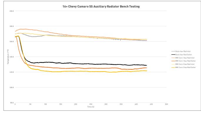
FIGURE 3: The stock radiator and both Mishimoto radiators were tested using identical inlet temperatures. Both Mishimoto cores showed an increase in heat transfer when compared to stock.
