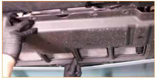
**06.** If equipped, remove the four nuts that secure the stock HD oil cooler to the underside of the vehicle. Slide the oil cooler off of the studs in order nuts]
