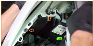
**13.** Remove the two screws that secure the bumper to the fender and loosen the inner screw. (3x 7mm screws)
