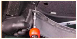
04. Remove the eight screws that secure the lower edge of the bumper. (8x 7mm screws)
