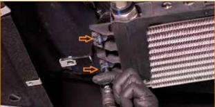
**07.** Place a drain bucket underneath the petcock on the radiator and use a pair of pliers to open the petcock. Remove the pressure cap from the expansion tank to expedite the draining process. Close the petcock on the radiator once all of the coolant has drained.
