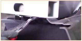
Remove the nut and two bolts that secure the auxiliary radiator assembly to the vehicle. Then remove the assembly from the vehicle and drain the excess coolant from the radiator. [1x 13mm nut, 2x 13mm bolts]
