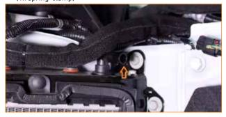
24. Compress the clamp that secures the outer hose to the radiator and slide the clamp down the hose. Remove the outer hose from the radiator. (1x spring-clamp)
