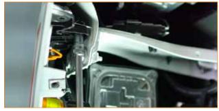
**14.** Pull the upper corner of the bumper away from the fender to release it from the vehicle.
