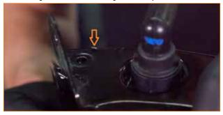
44. Secure the radiator to the upper section of the bracket with the provided bolts and washers. Then go back and tighten the outer bolts that join the brackets. (2x 10mm bolts, 2x washers)
