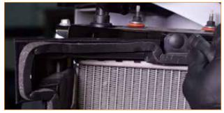
**25.** Remove the two clips that secure the rear duct to the radiator. Then remove the rear duct. (1x pop-clip, 1x tree clip)
