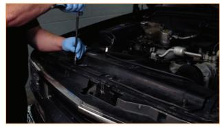
**3.** Remove the four 10mm bolts securing the upper cooling fan shroud to the lower cooling fan shroud.
