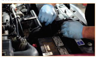
**9.** Install the three 10mm bolts holding the upper fan shroud to the radiator support.
