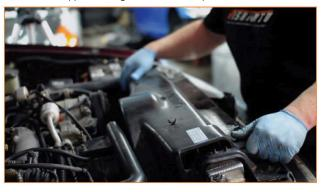
**8.** Install the four 10mm bolts securing the upper cooling fan shroud to the lower shroud.
