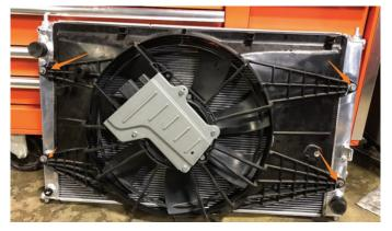
Remove the lower mounting bushings from the stock radiator and put into position in the lower radiator support.
