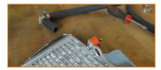
Cut the included hose to the recommended lengths. You need three separate hoses: 72 mm, 270 mm, and 660 mm.
