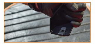
7. Install the small bracket to the studs on the firewall. (2x 10mm nuts)
