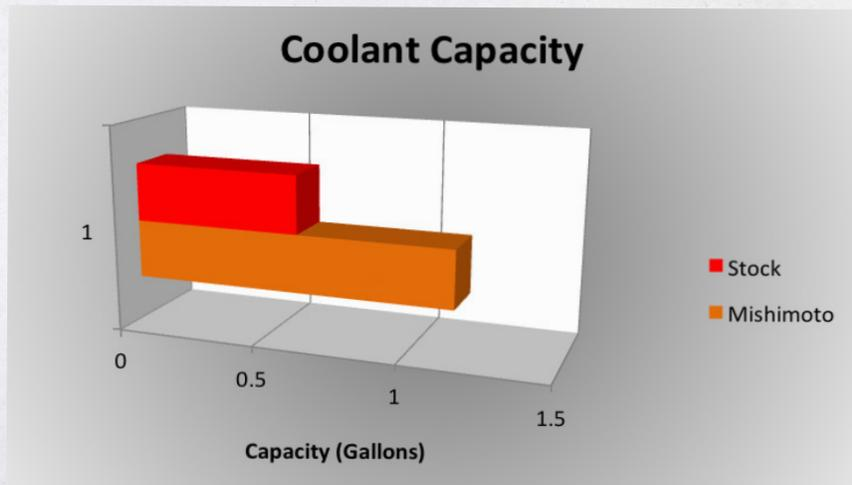
**Figure 6:** The stock M3 radiator holds 0.60 gal (2.27 L) of coolant, whereas the Mishimoto radiator holds 1.15 gal (4.35 L) of coolant, an increase over stock of 91%.
