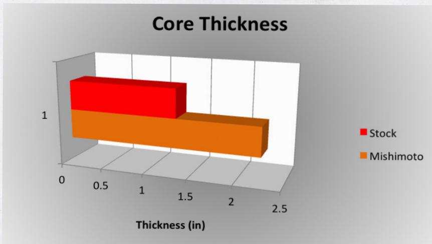
**Figure 5:** The stock radiator is 1.29 inches thick, whereas the Mishimoto radiator is 2.24 inches thick, an increase over stock of 73%.
