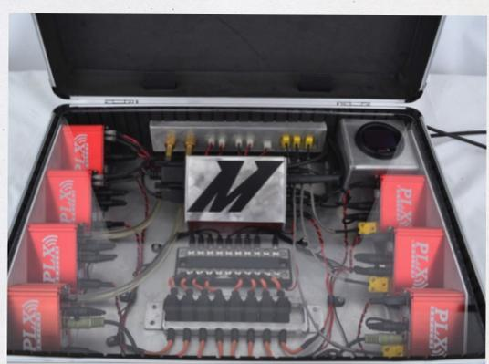
**Figure 1:** Fluid temperatures were taken from the inlet and outlet of both radiators using Mishimoto inline water temperature sensor adapters and PLX fluid temperature sensors. (Inlet sensor location is shown above.)
