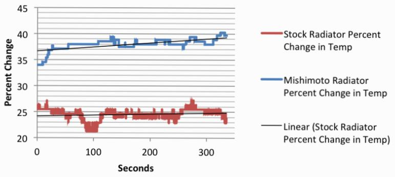
**Figure 11:** The chart above is a comparison of percent change in the outlet temperatures of the stock and Mishimoto radiators. The Mishimoto radiator has a 13% greater change in temperature than the stock radiator.
