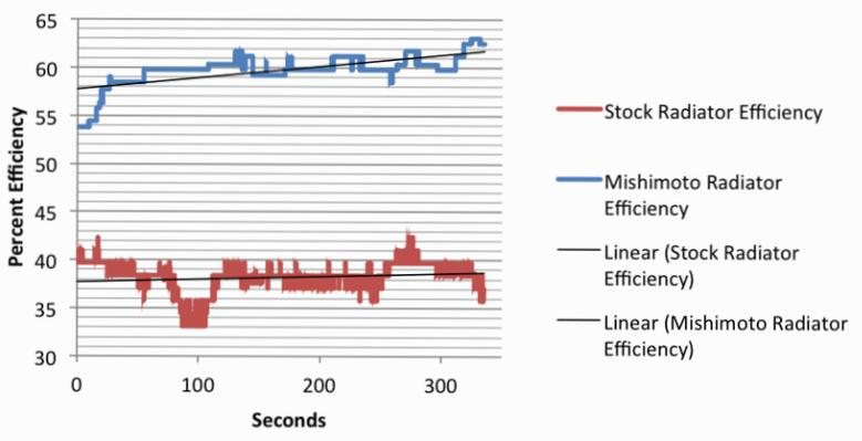
**Figure 10:** Comparison of efficiency between the stock and Mishimoto radiators. Notice that the Mishimoto radiator on average is approximately 20% more efficient than the stock radiator. This proves that the Mishimoto radiator has a higher capacity to keep the M3 running cooler.
