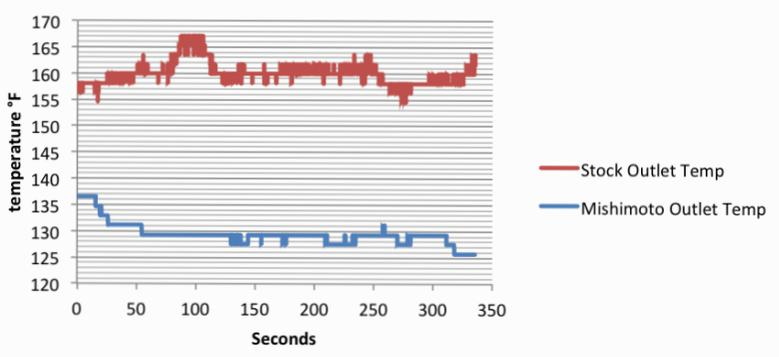
**Figure 9:** Comparison of radiator outlet temperatures measured from the stock and Mishimoto radiators. On average, the Mishimoto radiator outlet temperature was 30°F (16.7°C) less than the stock radiator outlet temperature.
