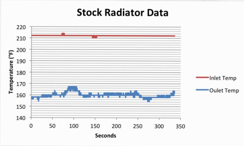
**Figure 7:** Highway test of stock radiator
