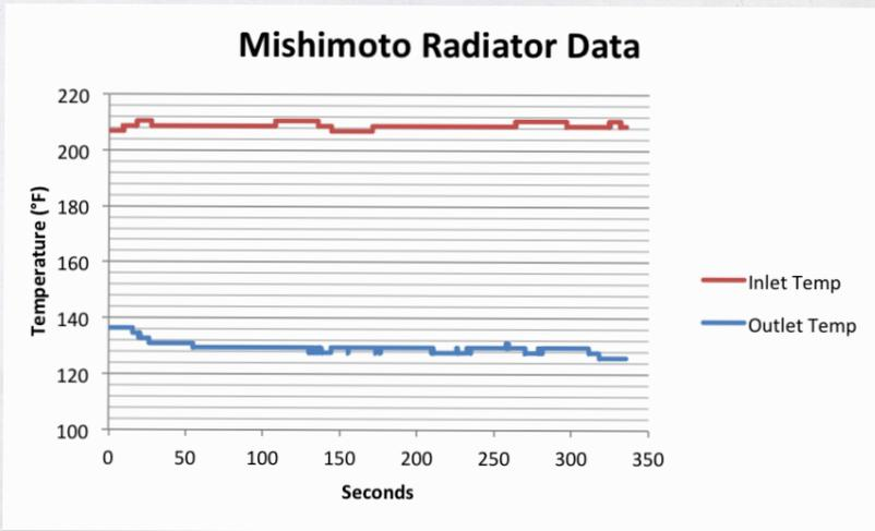
**Figure 8:** Highway test of stock radiator
