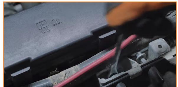
7. Release the clips that secure the nearby wiring to the fan. (2x tree clips)
