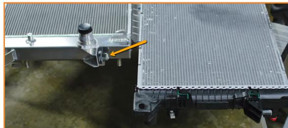
23. Using a 19mm wrench, tighten the drain plug on the Mishimoto radiator.
