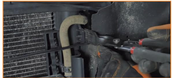
16. Optional Step: Using a hose clamp, pinch the upper transmission line.
