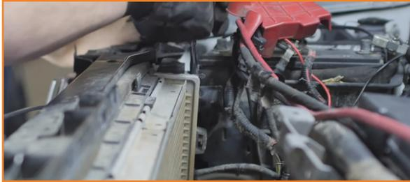
19. Separate the shrouding from the passenger side of the radiator. (4x pop-clips)
