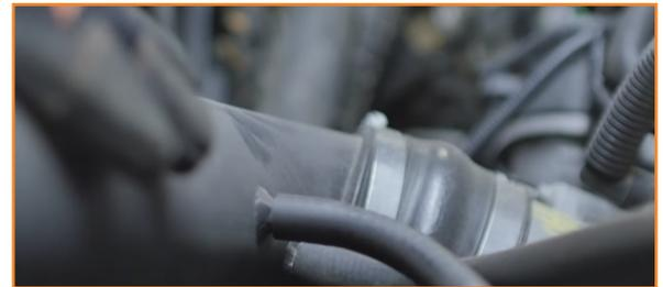
5. With all connections to the pipe free, remove your intake pipe.
