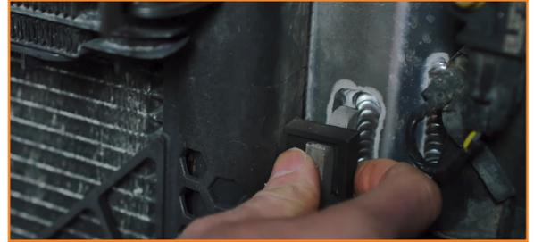
25. Using the two provided brackets, secure the passenger side of the AC condenser. (4x 4mm Allen screws)
