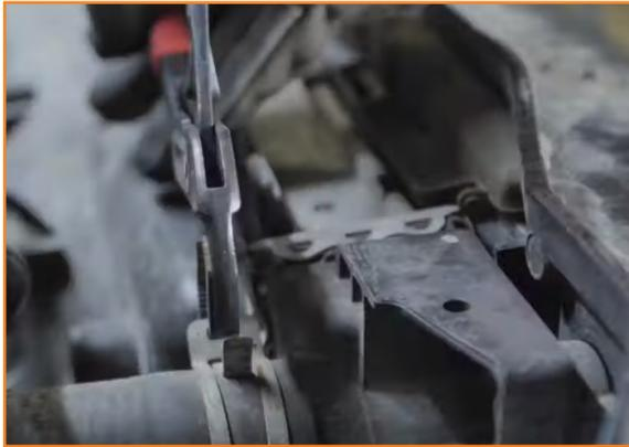
10. Remove the bolts that secure the fan shroud to the radiator. (2x 8mm bolts)
