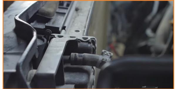
15. Release the shrouding connected to the driver side of the radiator. (2x pop-clips)
