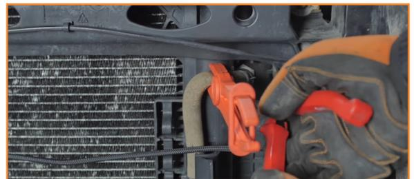
17. Remove the upper and lower transmission lines from the radiator. (2x spring clamps)
