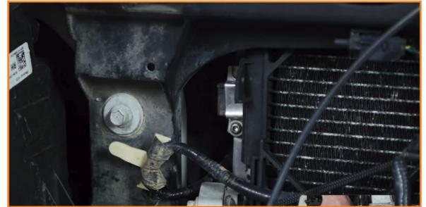
26. Attach the upper and lower transmission lines to the radiator. (2x spring clamps)
