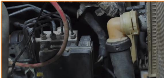
14. Compress the clamp on the overflow hose and slide the clamp down the hose. Then slide the overflow hose off the radiator. (1x spring clamp)
