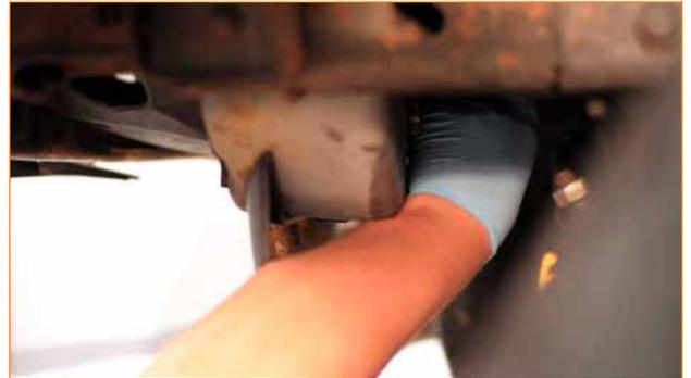
8. Remove the upper radiator stay brackets from the radiator support. Three 13mm bolts secure each bracket.
