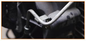
14. Remove the retaining clips from the transmission line adapter fittings on the radiator. Then remove the transmission lines form the adapter fittings.
