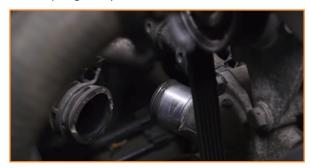
24. Install the Mishimoto lower radiator hose. (2x worm gear clamps)
