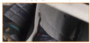
4. Remove the passenger-side lower splash shield. (1x pop-clip, 1x 7mm bolt)
