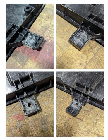
4. Secure the Mishimoto radiator to the top of the intercooler with provided brackets and M4 flange head fasteners as shown. The brackets are slotted to allow for a secure fit with the stock or the Mishimoto intercooler.
