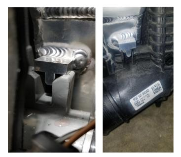
8. Slide the cooling fan down behind the radiator and engage the lower tabs with the hooks on the radiator. Use the two supplied M5 flange bolts to fasten the shroud to the radiator.
