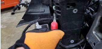
7. Note: it is normal for the lower T-mount feature on the radiator to appear too narrow for the slot in the intercooler. This is done by design to ensure fitment with both the Mishimoto intercooler as well as the stock intercooler.
