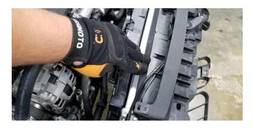
6. With the additional thickness of the Mishimoto radiator, it may be difficult to get the intercooler clips to snap into the core support. A tip for clipping the intercooler in place is to use a pry tool or pliers to hook the clip, then lever against the shroud to draw the clip through the hole. It does not take much force and the components are plastic, so take care when completing this step.
