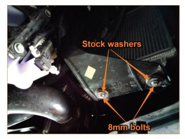
**03.** Install the Mishimoto DSG Cooler / Heat Exchanger using the stock washers and provided 8mm bolts. (2x 8mm bolts)
