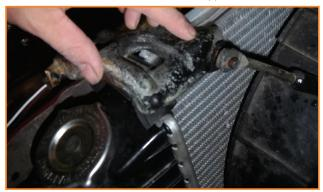
3. Remove the upper radiator brackets. (2 - 10mm bolts)
