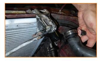
**5.** Remove the coolant over flow tube (near radiator cap) and the transmission cooler lines from the radiator as shown.
