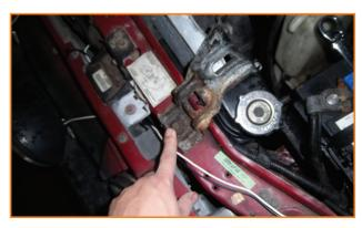
4. Remove the clamps and upper radiator hose and lower hose from the radiator.
