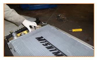
**2.** Install Mishimoto radiator into car making sure that the radiator is sitting on the OEM rubber mounts at the lower radiator support. Connect the automatic transmission lines as shown.
