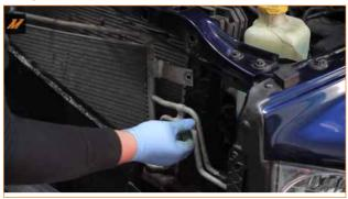
**21.** Remove the upper fan shroud. Lift upward on the shroud and push it toward the engine to unclip it from the lower shroud.
