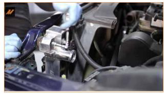
**8.** Reinstall the washer fluid reservoir. Reconnect the two electrical connections and secure the tank in place with two 13mm bolts.
