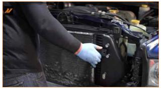
**15.** Move the AC condenser back to its proper position in front of the intercooler.
