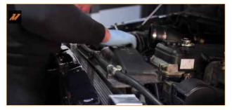
**5.** Using two 13mm bolts, reinstall the transmission cooler to the front of the radiator.
