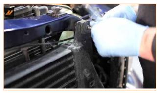
**8.** Remove the two T30 Torx bolts that secure the intercooler to the upper radiator support.
