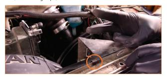
10. Remove the two bolts that secure the radiator to the support beam. (2x 10mm bolts)
