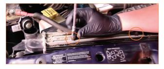
03. Place a drain pan or bucket under the petcock on the radiator. Loosen the petcock to drain the coolant from the radiator. Remove the radiator pressure cap to accelerate the draining process.
