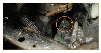
**04.** Compress the spring clamp that secures the upper radiator hose to the radiator and slide it down the hose, out of the way. Then remove the upper radiator hose from the radiator.
