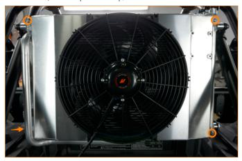
20. Install the fan shroud assembly to the primary radiator using hardware from the bag labeled "FAN SHROUD".  $(4x\ HF6X1.0-14)$
