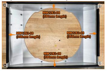
**18.** Install the weather stripping to the fan shroud as shown in the image above. (MM799, 2x MM1263-08 355mm length, and 2x MM1263-08 590mm length)
