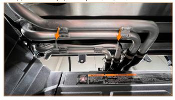
**56.** Route the Mishimoto fan controller wiring harness along the innermost pipe on the secondary radiator and loosely zip tie it in place. (2x zip ties)
