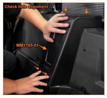
**36.** Test fit the center console cover to confirm the holes on the top and front align with the holes on brackets 6 and 7. Do not install the cover at this time. [MM1765-01]
