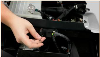
**62.** Turn the key to the accessory position, you should hear the fan turn on. Using a small flat head screwdriver, rotate the trimpot clockwise
