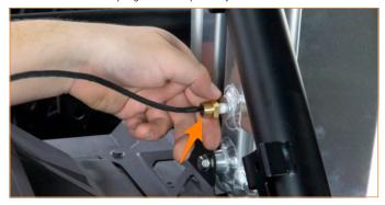
58. Apply Teflon tape to the Mishimoto fan controller temperature
