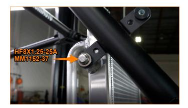
**13.** Loosely install the inner upper radiator brackets to the secondary radiator using hardware from the bag labeled "RADIATOR". (2x MM2384-03, 2x MM1152-37, and 2x HF8X1.25-25A)
