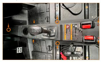
**37.** Remove the center console from the vehicle. (4x pop-clips, 3x Torx bolts)
