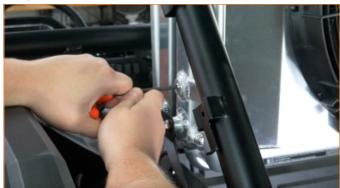
57. Remove the NPT plug from the primary radiator.
