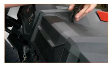
**38.** Remove the storage compartment from the top of the dashboard. (2x pop-clips)
