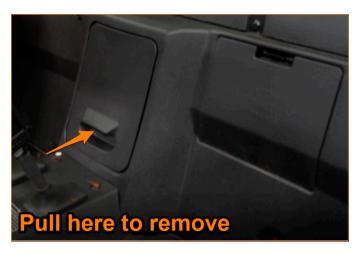
05. Remove the engine access cover.
