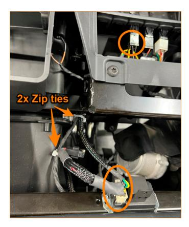
**47.** Connect the harness connectors to the Mishimoto fan controller and Mishimoto fan override switch then loosely zip tie the harness in place. \*Note, the zip ties used in this install guide are white in color to make them easier to see in the images. The zip ties supplied with the kit will be black in color. (2x zip ties)
