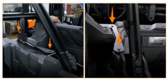
**11.** Install the lower radiator bracket assemblies into the existing holes just in front of the rear roll bar mounts.
