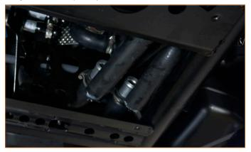
**34.** The image above shows the primary radiator coolant hoses after being cut to the correct length.
