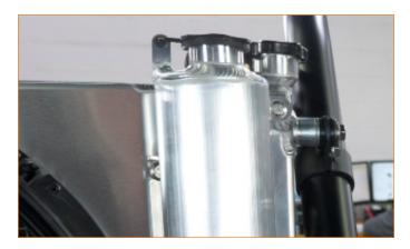
21. Fasten the coolant reservoir to the fan shroud using hardware from the bag labeled "RESERVOIR". (4x HF6X1.0-10B)
