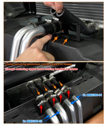
25. Install coolant pipes 1 and 2 into hoses 6 and 7 using the provided clamps. The clamps furthest away from the ends of the hoses are used to seal the connection. The clamps closest to the ends of the hoses are to be placed over the tines on the upper hose routing bracket. Once
