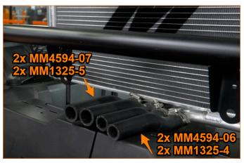
23. Connect the short sides of hoses 6 and 7 to the primary and secondary radiators using the provided clamps. [2x MM4594-06, 2x MM4594-07, 2x MM1325-4, 2x MM1325-5]
