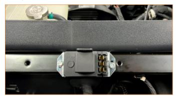
**42.** Secure the Mishimoto fan controller in place with the provided self-tapping screws. DO NOT USE AN IMPACT DRIVER ON THE SELF-TAPPING SCREWS. (Mishimoto fan controller, 2x self-tapping screws)
