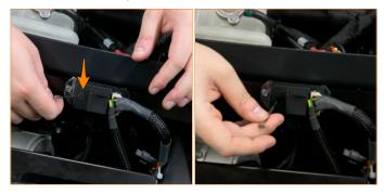
**48.** Remove the rubber plug covering the fan activation trimpot. Using a small flat head screwdriver, rotate the trimpot counterclockwise to its
