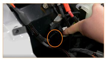
**45.** Feed the short end of the Mishimoto fan controller wiring harness through the hole in the front bulkhead and then reinstall the grommet. (Mishimoto fan wiring harness)
