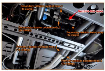
**02.** Remove the two primary radiator coolant hoses and two secondary radiator coolant hoses from the aluminum pipes under the rear of the vehicle. Have a drain pan ready and remove the hoses slowly as this is how the cooling systems must be drained. Once drained, remove the secondary radiator coolant hose from the water pump. (5x spring clamps, 1x hose)
