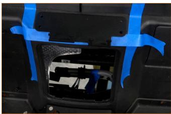
**07.** Place the lower hose routing bracket on the rear bulkhead and position it centered between the tape lines. (MM2384-07)
