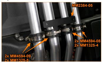
26. Secure the coolant pipes and bracket 5 in place using the provided insulators and clamps. Be sure to place the clamps over the tines on the lower hose routing bracket and bracket 5. Pay close attention to how the clamps are oriented in the image above. [MM2384-05, 2x MM4594-08, 2x MM4594-09, 2x MM1325-4, and 2x MM1325-5]
