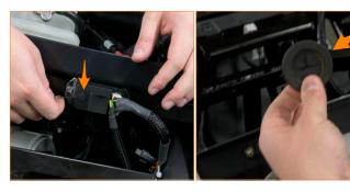
43. Remove the grommet from the front bulkhead.
