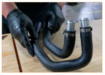
**31.** Insert 1x pipe 4 into the short ends of both Mishimoto hose 3 and Mishimoto hose 4, then secure the pipes in place using the provided worm gear clamps. (MM4594-03, MM4594-04, 2x MM2386-04, and 2x MM1325-5)
