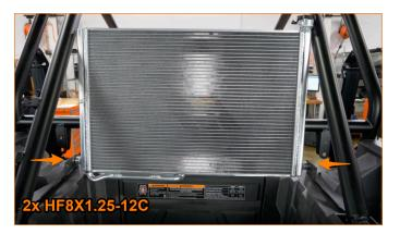
**12.** Place the secondary radiator between the two lower radiator bracket assemblies and loosely fasten it in place using hardware from the bag labeled "RADIATOR". [MM5235 and 2x HF8X1.25-12C]
