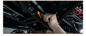
53. Feed the Mishimoto fan controller wiring harness up into the cabin,
