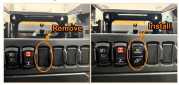
**46.** Remove the blank switch plate from the center of the dashboard and install the Mishimoto fan override switch in its place. (Mishimoto fan override switch)
