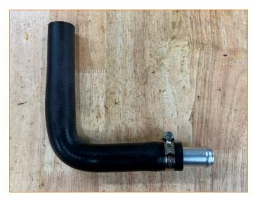
**27.** Insert pipe 3 into the shorter end of hose 1 then secure it in place using one of the provided worm gear clamps. (MM2386-03, MM4594-01, and MM1325-4)
