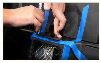
**08.** Transfer the lower hose routing bracket mounting holes onto the rear bulkhead using a marker. Using a drill and 1/4" drill bit, drill a hole at each of the markings, then remove the painters' tape. (Marker, drill, and 1/4" drill bit)
