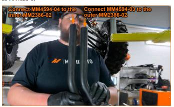
**32.** Connect Mishimoto hose 4 to the innermost pipe 2 then secure it in place with one of the provided worm gear clamps. Connect Mishimoto hose 3 to the outermost pipe 2 then secure it in place with one of the provided worm gear clamps. (2x MM1325-5)
