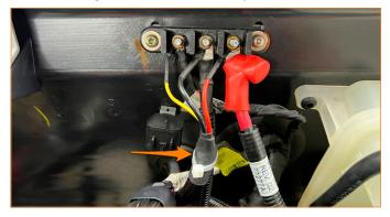
**50.** Connect the positive, ground, and accessory wires from the Mishimoto fan controller wiring harness to the power distribution bar. Zip tie the harness in place. (1x zip tie)
