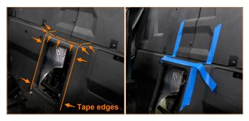
**06.** Apply painters' tape as shown in the above images. The tape will be used as a guide for locating one of the included brackets.
