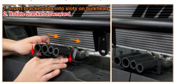
**24.** Install the upper hose routing bracket into the slots located on the top surface of the rear bulkhead.
