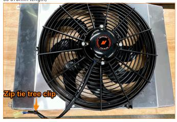
19. Fasten the fan to the fan shroud as shown in the image above using hardware from the bag labeled "FAN SHROUD". Secure the fan wiring harness to the fan shroud using 1x zip tie tree clip. (MM1301, 4x HF6X1.0-12A, and 1x zip tie tree clip)
