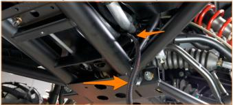
**52.** Feed the long end of the Mishimoto fan controller wiring harness down towards the ground between the aluminum coolant pipes.
