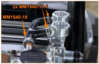
22. Install hose 5 to the two radiator overflow ports and the coolant reservoir port. Secure it in place using the provided spring clamps. [MM4594-05, 2x MM1540-17.4, and MM1540-19]
