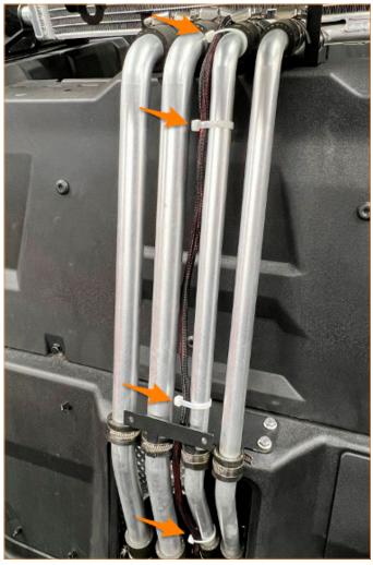
**55.** Route the Mishimoto fan controller wiring harness along the innermost pipe 1 and loosely zip tie it in place. (4x zip ties)
