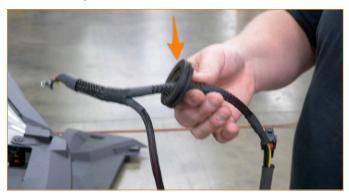
**44.** Slide the grommet over the Mishimoto fan controller wiring harness and into the position shown in the image above. (Mishimoto fan wiring harness)
