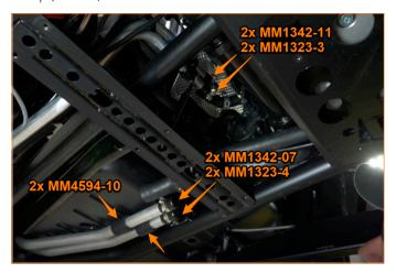
03. Slide the MM4594-10 grommets over the primary radiator coolant pipes until they're in the location shown in the image above. Install the rubber caps over the ends of the primary radiator coolant pipes and secondary radiator coolant pipes and secure them in place with the
