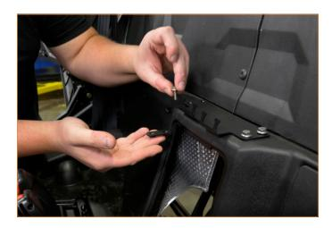
**09.** Secure the lower hose routing bracket in place using the provided hardware from the bag labeled "HOSE ROUTING" and 2x nut brackets. [MM2384-07, 2x MM2384-08, and 4x HF6X1.0-16D]
