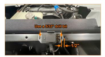
41. Place the Mishimoto fan controller on the upper bar located just behind the front bulkhead and space it approximately 1/2" from the existing hole shown in the image above. Transfer the location of the two mounting holes on the Mishimoto fan controller to the bar using a marker. Remove the Mishimoto fan controller from the bar and drill a 5/32" hole at the two marked locations. (Mishimoto fan controller, marker, 5/32" drill bit)
