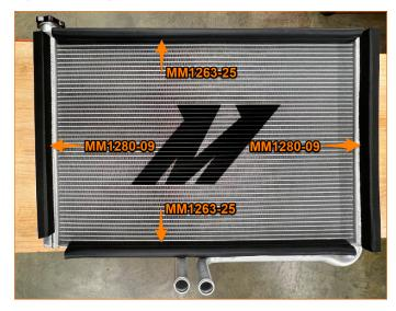
14. Install the weather stripping and adhesive-backed foam to the front of the primary radiator as shown in the image above. (MM5234, 2x MM1280-09, and 2x MM1263-25)
