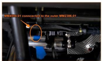
29. Connect the Mishimoto hose 1 assembly to the outermost pipe 1 and secure it in place with one of the provided worm gear clamps. [1x MM1325-4]
