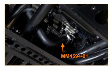
28. Connect the Mishimoto hose 1 assembly to the secondary radiator coolant hose 1 and secure it with one of the provided worm gear clamps. [1x MM1325-4]
