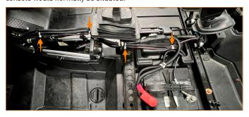
**54.** Route the Mishimoto fan controller wiring harness along the existing vehicle wiring harness and loosely zip tie it in place. (4x zip ties)
