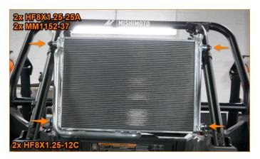
**15.** Place the primary radiator between the two lower and upper radiator bracket assemblies and loosely fasten it in place using hardware from the bag labeled "RADIATOR". (MM5234, 2x HF8X1.25-12C, 2x HF8X1.25-25A, and 2x MM1152-37)
