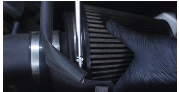
17. Loosen the clamp on the filter within the housing, and then separate the filter from the pipe. (1x worm gear clamp)
