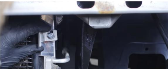
39. Connect the radiator stays to the Mishimoto radiator and secure them to the vehicle's frame using the original hardware. (2x 10mm bolts and washers)
