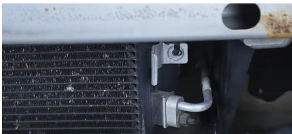
14. Remove the bolts that secure the AC condenser to the radiator, which includes the two radiator stays located on the top brackets. (4x 10mm bolts)
