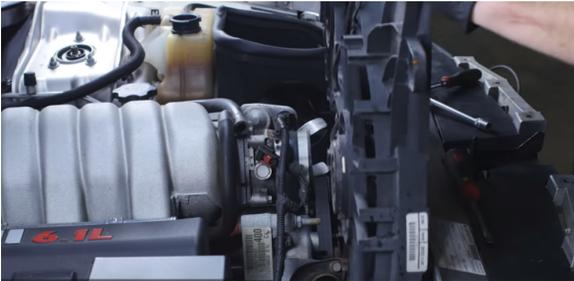
24. Compress the clamp that secures the outer hose to the radiator and slide it down the hose. Separate the lower radiator hose from the radiator. These connections are often tight so you may need to use a pick to separate the hose, but be careful not to cause any damage. (1x spring clamp)
