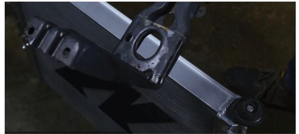
29. If you are installing MMRAD-SRT-09, you might need to attach the provided bracket, two bolts, two washers, and one spacer depending on your AC condenser. This attaches to the top right of the radiator when looking at it from the front. For the MMRAD-SRT-15, you may need to attach the bracket, two bolts, two washers, and long bolt included in your kit depending on your AC condenser. These hardware pieces attach to the upper right of the radiator when looking at it from the front.
