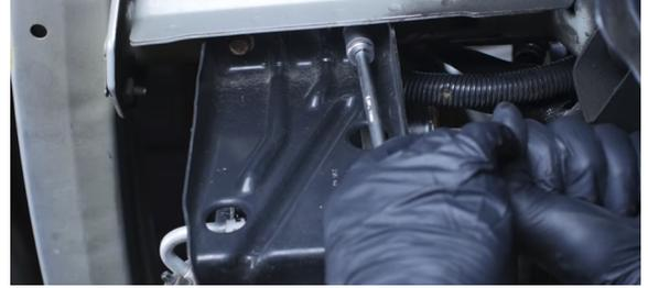
27. Lower the radiator from the vehicle. Due to the radiator's size and the position of the AC condenser, it will be useful to have someone else on hand to help with this step.
