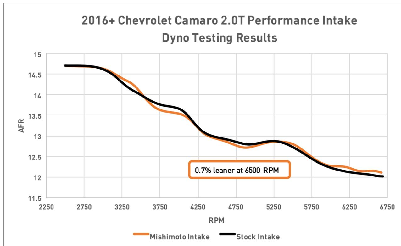
FIGURE 4: Dyno results (air/fuel ratio)
