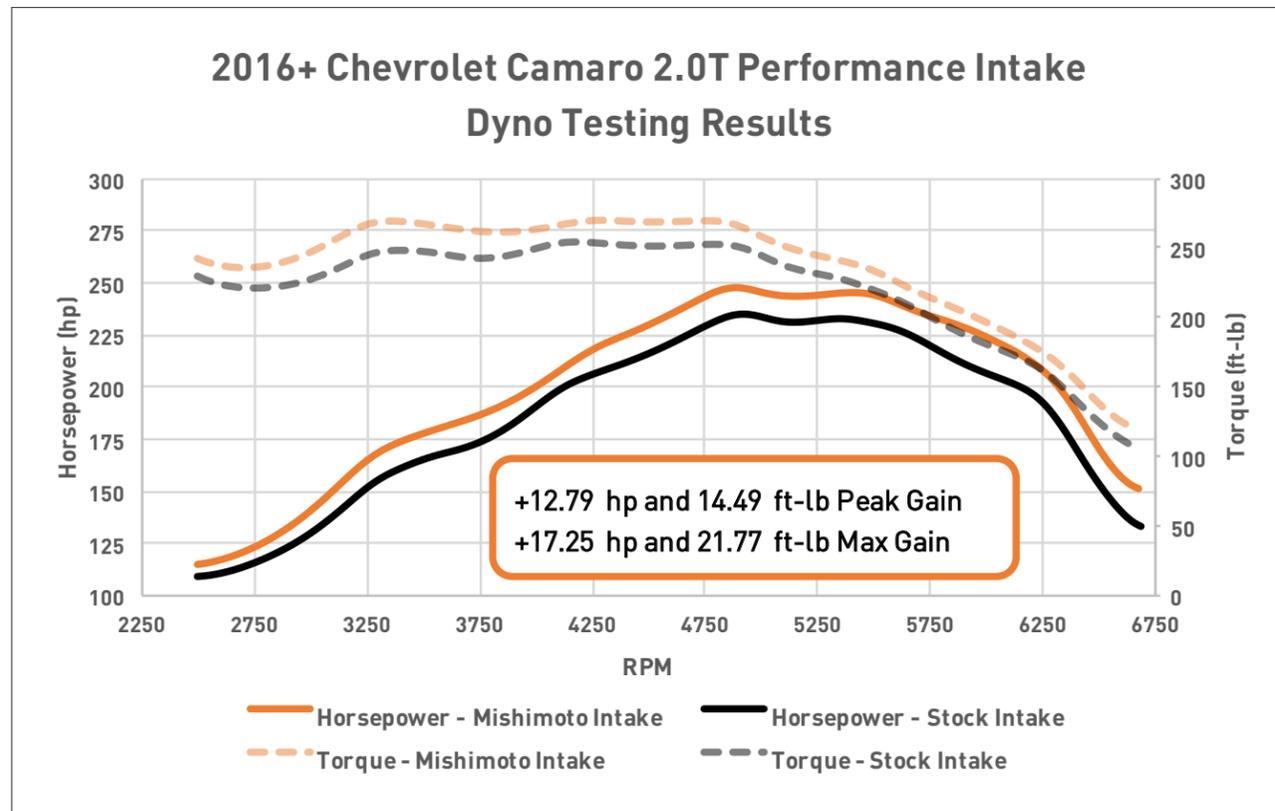
FIGURE 5: Dyno results (horsepower and torque)
