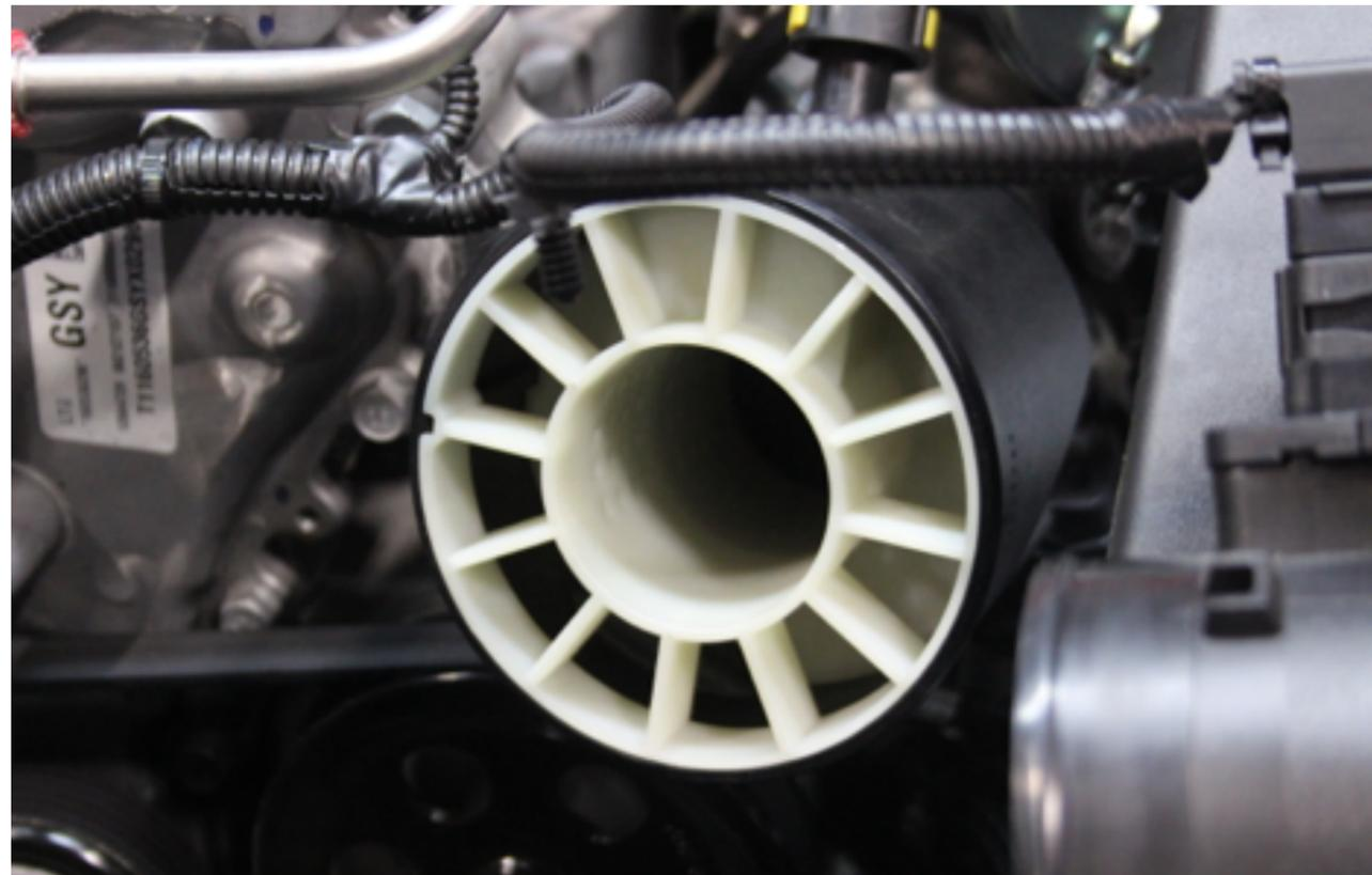
FIGURE 1: Sound "muffler" located inside stock intake hose.
