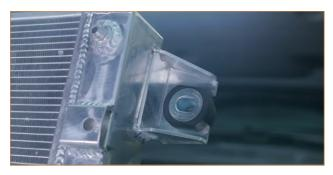
25. Remove the five clip nuts from the stock radiator, and transfer them to the Mishimoto radiator. Use a screwdriver to bend the tang on the clip nut to retain it on the radiator. (5x clip nuts)
