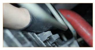
10. Remove the five bolts that secure the fan shroud to the radiator. (5x 8mm bolts)
