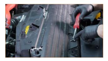
09. Separate the transmission cooler lines from the clips that secure them to the fan shroud.
