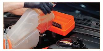
**05.** Once you have drained the coolant below the port at the bottom of the expansion tank, pinch off the coolant hose, compress the clamp that secures it, and separate the hose from the tank. Now remove the tank from the vehicle and drain the remaining coolant.
