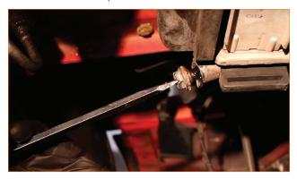
**02.** Remove the coolant bleeder screw from the top of the stock expansion tank.
