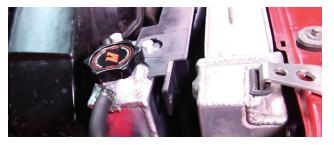
13. Attach the overflow hose to the port on the expansion tank, and then secure the hose with the worm-gear clamp.
