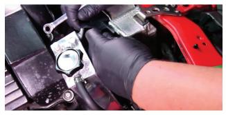
12. Slip the forward mounting peg on the top of the Mishimoto expansion tank into the hole where the bleeder screw seal was removed.
