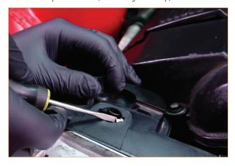
**05.** Disconnect the electrical harness from the coolant level sensor, located on the bottom of the expansion tank.
