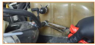
4. Pull out the clip that secures the upper radiator hose to the radiator. Slide the upper radiator hose off the radiator. You need to move the hose out of the way so you can successfully lift the battery tray. (1x spring clip)
