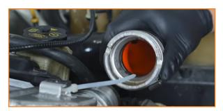
5. Pull off the vacuum lines clipped to the reservoir tank.
