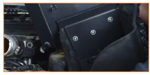
17. Install the included bracket to the expansion tank. (2x 5mm Allen bolts)
