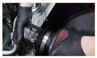
15. Install the CNC-machined fitting to the port on the Mishimoto induction hose, and secure it with the small worm gear clamp provided with the kit. Then slip the remaining worm gear clamps over each end of the induction hose. (3x worm gear clamps)
