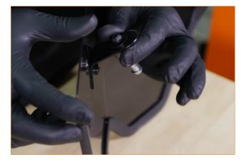
06. Install the last mounting peg to the bracket with the M cutout using a long bolt, lock washer, and large flat washer. Then install the bracket to the airbox with a pair of short bolts, lock washers, and small flat washers. Tighten the bracket mounting bolts completely. (1x long Allen bolt, 1x large washer, 2x short Allen bolt, 2x small flat washer, 3x lock washers)
