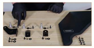
02. Locate the bracket in your kit that has a small tab. Install this bracket to the airbox so that the tab slides into the slot on the airbox. Then secure the bracket with one of the short Allen bolts, a lock washer, and one of the small flat washers. (1x short 4mm Allen bolt, 1x lock washer, 1x small flat washer)
