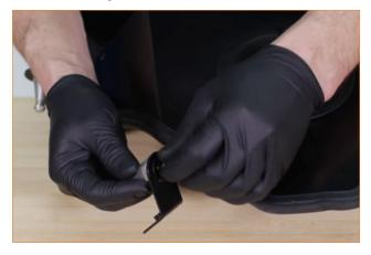
05. Install a lock washer and small washer over one of the short Allen bolts. Then install the small bracket to the inside of the airbox as shown here. Leave the bolt slightly loose for now. (1x short 4mm Allen bolt, 1x lock washer, 1x small flat washer)
