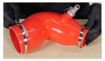
16. Install the Mishimoto induction hose to the MAF housing and the turbocharger inlet. Turn the MAF housing until the sensor is pointed upward, and ensure that the housing is pressed against the airbox seal. Adjust the hose clamps until they sit over the bead roll of the connection, and then tighten them to secure the hose. Then reconnect the MAF sensor.
