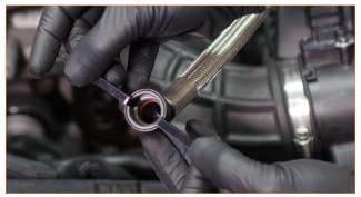
**08.** Disconnect the electrical harness from the mass airflow (MAF) sensor, and separate the harness from the intake tube. To release this connector, slide the red locking tab up, and then depress the black tab.
