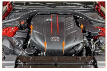
02. Remove the airbox and intake tube.
