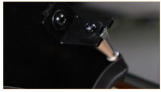
09. Compress the spring clamp that secures the sound generator tube to the induction hose, and pull the sound generator tube off the port. The plastic elbow will remain in the induction hose.
