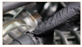
10. Loosen the worm-gear clamp that secures the induction hose to the throttle body. Then pull the induction hose off the throttle body.
