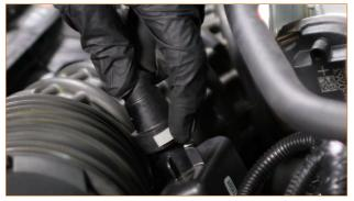
**12.** Loosen the worm-gear clamp that secures the induction hose to the stock airbox. Then remove the induction hose from the vehicle.
