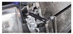
8. Compress the clamp securing the cooler line to the transmission cooler and slide the hose off the port. Again, use rubber plugs to prevent unnecessary spillage. (1x spring clamp)
