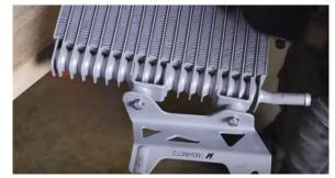
12. Install the Mishimoto transmission cooler. Position the top of the cooler brackets underneath the two tabs on the radiator. Secure the brackets with the provided hardware. If you have a Mishimoto rad installed, place the spacer behind the bracket.
