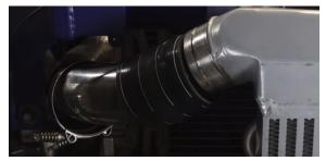
3. Loosen the clamps on the coupler between the intercooler and cold-side pipe. Slide the coupler off the intercooler end tank. (2x t-bolt clamps)
