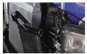
Loosen the clamps on the coupler between the intercooler and hot-side pipe. Slide the coupler off the intercooler end tank.
