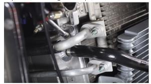
16. Reinstall the hose to the port on the bottom of the transmission cooler. Secure the connection with the clamp still on the hose. (1x spring clamp)
