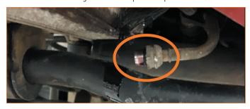
07. Install the MM1513-15 fitting into the stock liquid-to-liquid transmission. Install the stock transmission cooler fitting into the MM1670 adapter. \*\*Inspect the O-ring on the stock transmission cooler fitting. Replace it with the provided O-ring if it is damaged.\*\*
