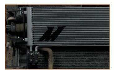
09. Trim the back of the grille support as shown in the above image. This must be done to add clearance around the MM1661 line assembly.
