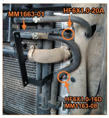
05. Install the transmission cooler to brackets using the provided hardware. (4x HF6X1.0-14)
