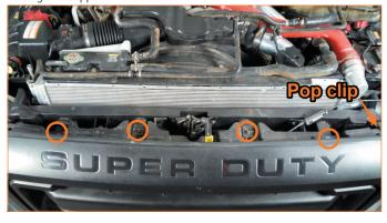
02. Remove the headlights, then remove the grille support. (6x 10mm bolts and 4x 13mm bolts)
