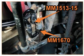
08. Install the MM1661 line assembly and connect it to the MM1513-15 fitting, MM1670 adapter, and the transmission cooler using the provided worm gear clamps. (4x MM1325-2)
