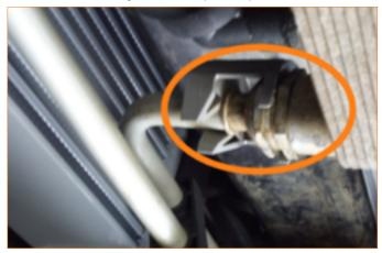
Remove the metal transmission lines from the plastic line separator and plastic line fitting clip. Rearrange the lines to resemble the above image and then reconnect the metal transmission lines to the plastic line separator and plastic line fitting clip.
