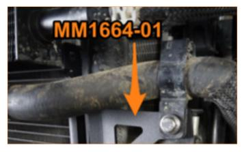
**08.** Install the MM1664-02 bracket to the secondary radiator using the provided hardware. (2x HF6X1.0-20A)
