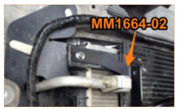
**09.** Install the transmission cooler to brackets using the provided hardware. (4x HF6X1.0-14)
