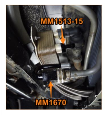
Install the MM1662 line assembly and connect it to the MM1513-15 fitting, MM1670 adapter, and the transmission cooler using the provided worm gear clamps. (4x MM1325-2)
