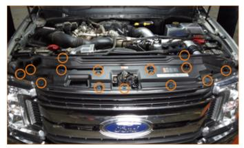
**02.** Remove the front grille. (8x 10mm bolts) - once bolts are removed pull outward on the grille to unseat it from the grille support.
