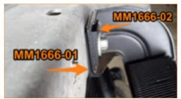
07. Install the MM1664-01 bracket between metal tube mount and the secondary radiator using the provided hardware. (1x HF6X1.0-20A)
