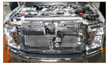
**04.** Remove the grille support. (4x 10mm bolts, 4x 13mm bolts, 6x tree clips, 1x electrical harness and electrical connector)
