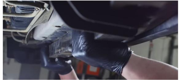
3. Separate the shrouding that was behind the support beam. (8x pop-clips)
