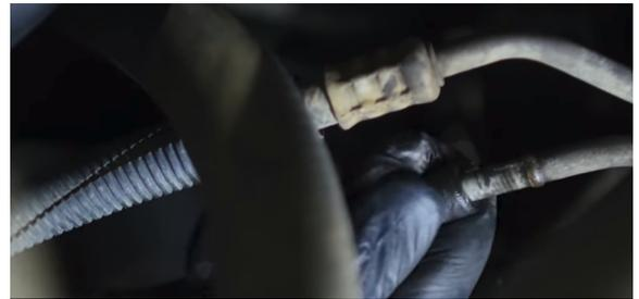
10. Slide the second transmission hose off the line as shown here. We recommend plugging this line to limit the leakage.
