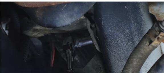
17. Secure the top brackets on the transmission cooler. You can reach underneath the grille with a long extension to get to the brackets. Make sure the metal tabs are set behind each bracket. (2x 8mm bolts)
