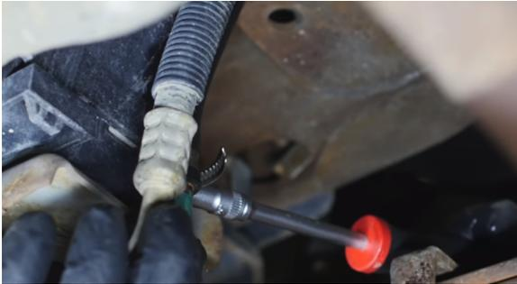
23. Secure the transmission cooler hoses with the plastic fasteners.
