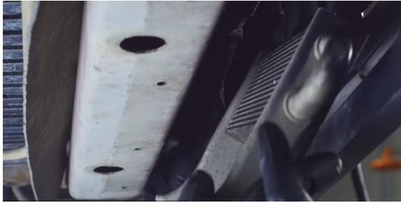
5. Remove the bolts that secure the transmission cooler.
