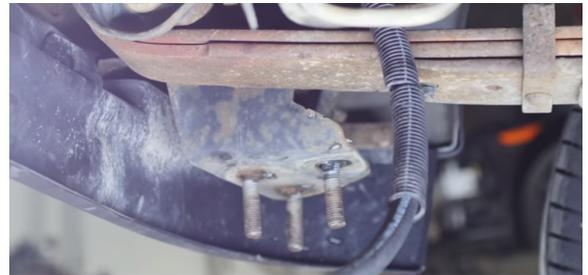
21. Install your second hose to the driver-side port on the transmission cooler. Then feed the hose up past the cooler and along the edge toward the transmission line. (1x worm gear clamp)
