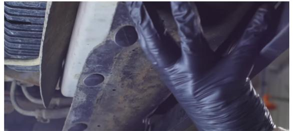
4. Remove the bolts that secure the power steering cooler. Once free, gently lower the cooler and let it rest in place or prop it up while moving onto the next steps.
