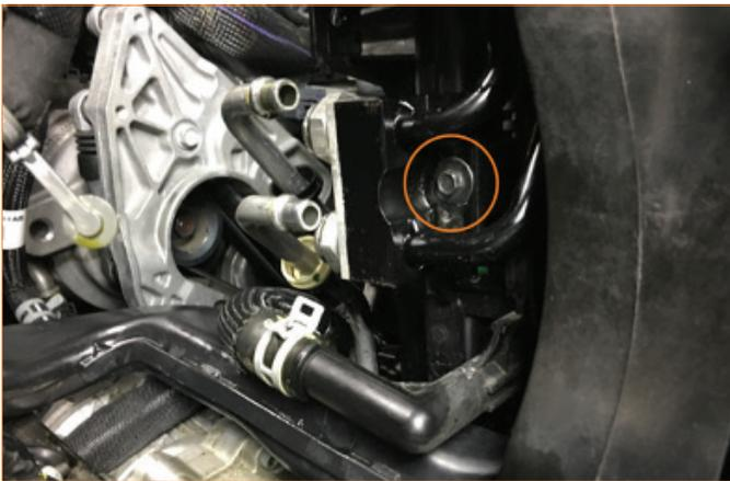
13. Pull back on the tab located on the driver side of the radiator that secures the transmission cooler to the radiator and remove the transmission cooler from the vehicle.
