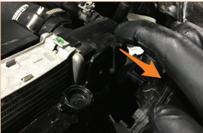
14. Remove the bolts that secure the horn brackets to the radiator support (2x 10mm bolts) and replace them with provided allen bolts (2x 4mm allen bolts).
