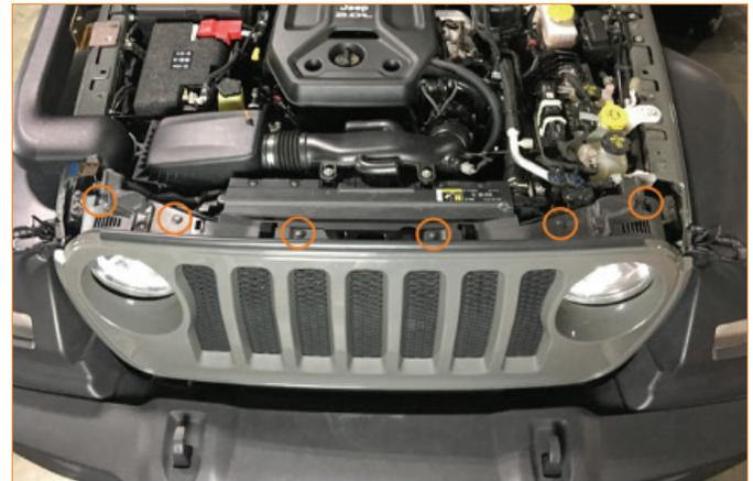
**02.** Pull outward on bottom of grille to remove it from the vehicle.
