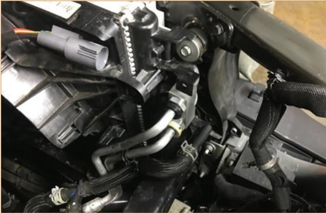
20. Reinstall the passenger-side headlight (3x 10mm bolts and 1x electrical harness).
