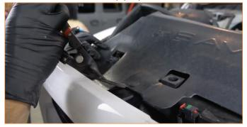
03. Remove the bolts screws that secure the grille. (4x 10mm screws)
