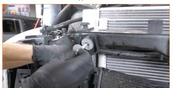
**20.** Reinstall the AC condenser, including the brackets on the driver side. (2x 10mm bolts, 2x 13mm bolts)
