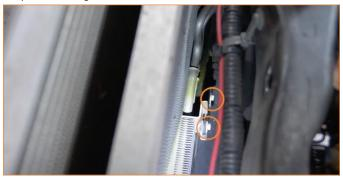
10. Remove the bolts that secure the transmission cooler. (2x 10mm bolts)
