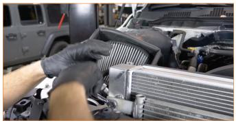
**11.** Pull the spring clip on the passenger-side transmission cooler line. Pull the loosened line out of the transmission cooler. (1x spring clip)
