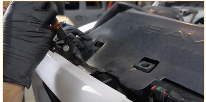
**03.** Remove the bolts screws that secure the grille. (4x 10mm screws)
