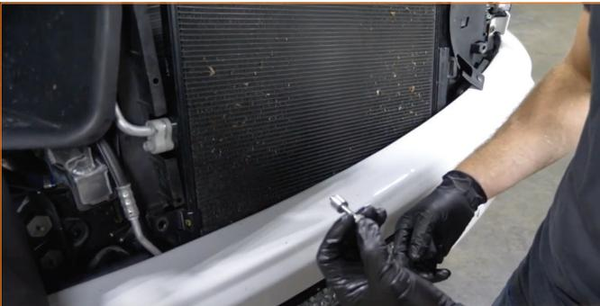
**19.** Once through those holes, position the spacer on the bolt, and finally secure the bolt to the vehicle. (2x 10mm bolts, 2x spacers)
