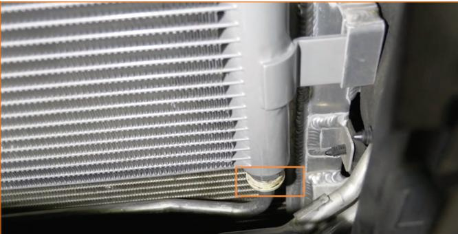
**18.** On each side of the cooler, use the provided long bolt and place it through the two upper holes on the power steering cooler.
