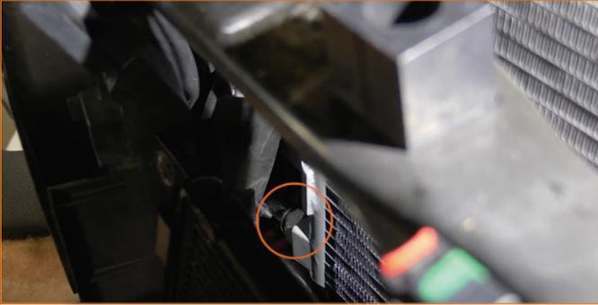
**17.** Attach the cooler line to the transmission cooler on the driver side. Be sure to set the dust boot over the connection. (1x spring clip)
