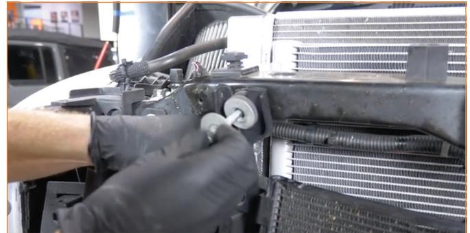
**22.** Reinstall the AC condenser, including the brackets on the driver side. (2x 10mm bolts, 2x 13mm bolts)
