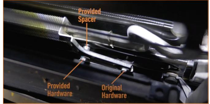
**21.** Reinstall the AC condenser support. (1x 13mm bolt)
