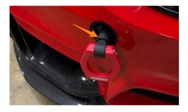
**11.** Tighten socket head cap screw securing the tow hook in desired position.
