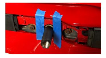
**06.** Put one piece of painter's tape horizontally above and below the tow hook. Put a final piece of tape horizontally on top to keep the tape together. Remove the tow hook shaft with 19mm wrench. (View top left image on next page)
