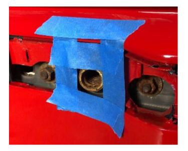
**07.** Raise the tape assembly (do not remove) and reinstall the tow hook cover using the top piece of tape as a "hinge". Place the tape back in its original position but over the tow hook cover. Mark the center of the square where the center of the tow hook shaft was located with a marker or center punch. (View top right image)
