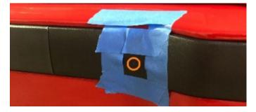
**08.** Remove the tow hook cover and drill where marked in step 7 to approximately 1". Reinstall tow hook cover and test fitment of tow hook shaft. It may be necessary to enlarge the hole slightly. Tighten tow hook shaft.
