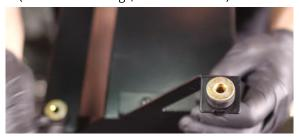
12. Install the supplied rubber mount to the threaded hole on the inside of the radiator support. (1x rubber mount)
