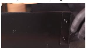
11. Install the bushings and metal inserts to the Mishimoto airbox.(2x rubber bushings, 2x metal inserts)
