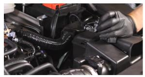
3. Loosen the clamp that secures the intake tube to the turbocharger inlet pipe. Then, separate the tube from the turbocharger.
