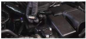
2. Compress the clip that holds the wiring to the airbox to separate the two.
