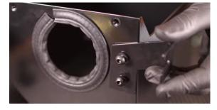
10. Install the large bracket to the bottom of the airbox. (2x 4mm Allen bolts, 2x large washers)
