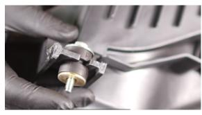
6. Separate the MAF sensor from the airbox. Two screws hold it in place. (2x Phillips head screws)
