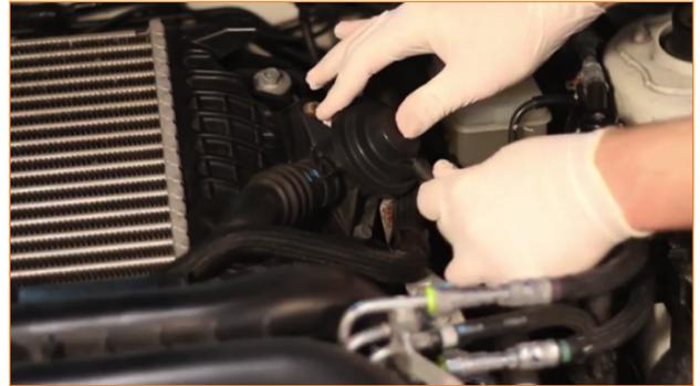
2. Remove the two 10mm bolts holding the bypass valve in place.
