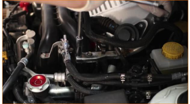
6. Install the two 12mm bolts for the turbo inlet, and then torque the bolts to 15 ft-lb.
