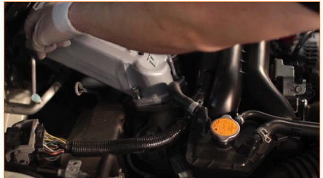
7. Using the two 10mm bolts you removed earlier, reinstall the bypass valve.
