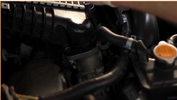
7. Lift and remove the stock intercooler.
