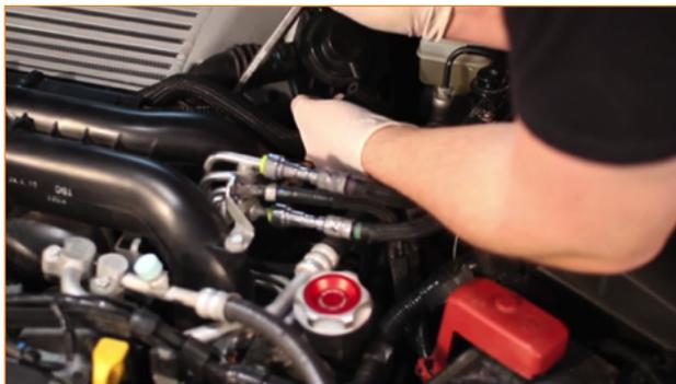
5. Reinstall the intercooler mounting bracket by installing the longer 12mm bolt at the intercooler first, and then the two smaller 12mm bolts on the intake manifold.
