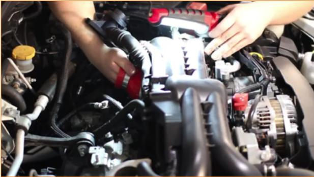
2. Install the Mishimoto intercooler, leaving the intercooler-to-throttle body hose slightly loose.
