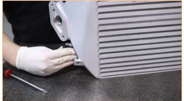
2. Install the supplied rubber gasket onto the inlet flange on the Mishimoto intercooler.
