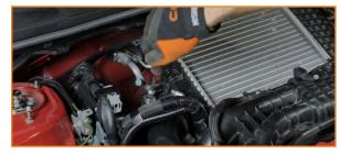
4. Remove the bolts on the intercooler bracket, located on the driver side. (2x 12mm bolts)
