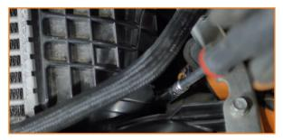
3. Remove the bolts that secure each side of the intercooler. (2x 12mm bolts)
