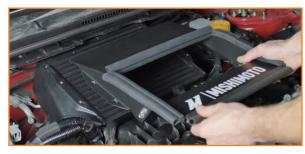
18. Install the shrouding to the face of the intercooler. Align the holes on the bracket with those on the intercooler. (4x 4mm Allen bolts)
