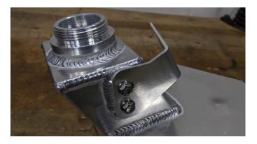
**14.** Install Mishimoto coolant tank using the hardware from the stock coolant tank removed in step 11 and the 3x mounting locations shown.
