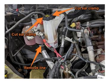
10. Disconnect coolant level sensor.
