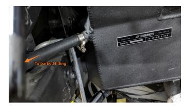
**16.** Run supplied hose from engine side coolant fitting to Mishimoto expansion tank.
