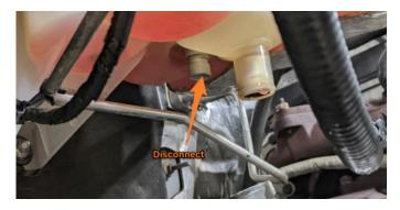
11. Remove stock coolant tank.
