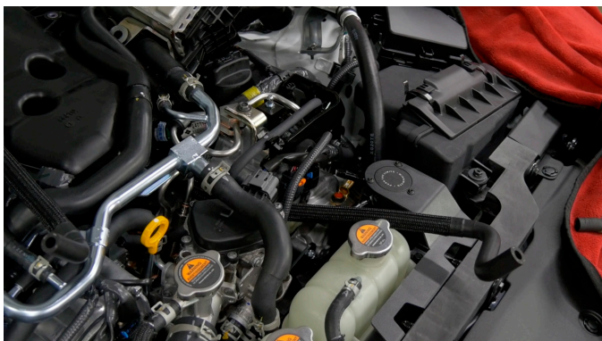
10. Install the catch can outlet hose. This is the longer hose with 2x 90-degree bend on one end. Feed it in between the intercooler and the manifold, as shown. Place this hose into the plastic clip, connect it to the manifold port and secure it with a worm gear clamp.
