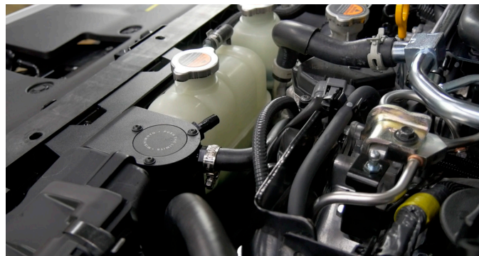
11. Connect the other end of the outlet hose to the catch can outlet port, secure with a worm gear clamp.
