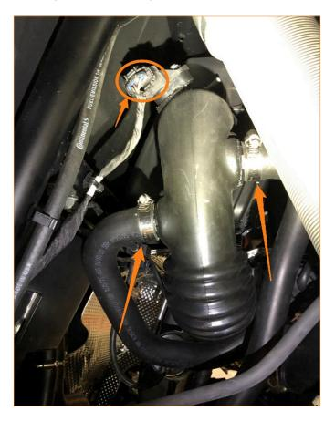
04. Remove the intake pipe from the vehicle through the wheel well.
