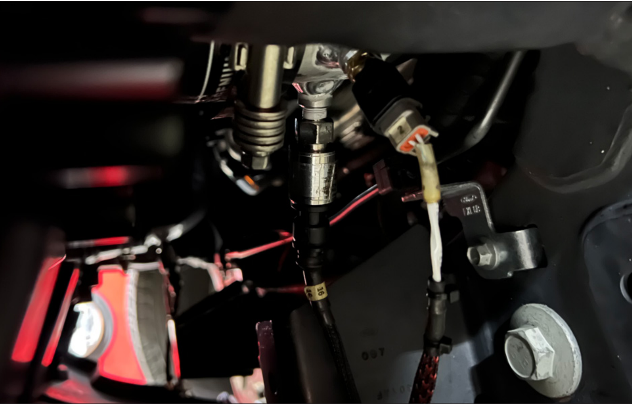
Figure 4: Pressure and Temperature Sensors Installed in the Cold-Side Intercooler Piping
