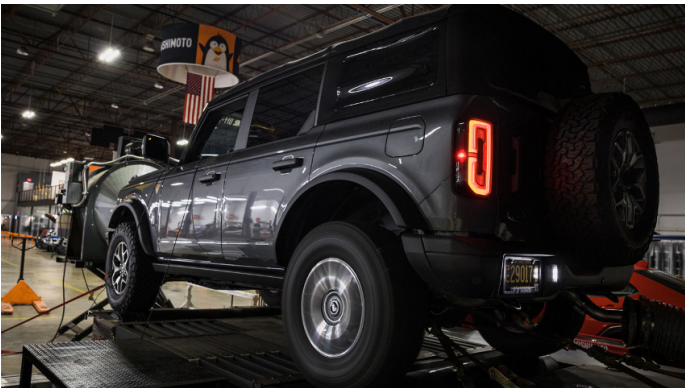
Figure 7: A DynoJet dynamometer was used for 2.7L testing.
