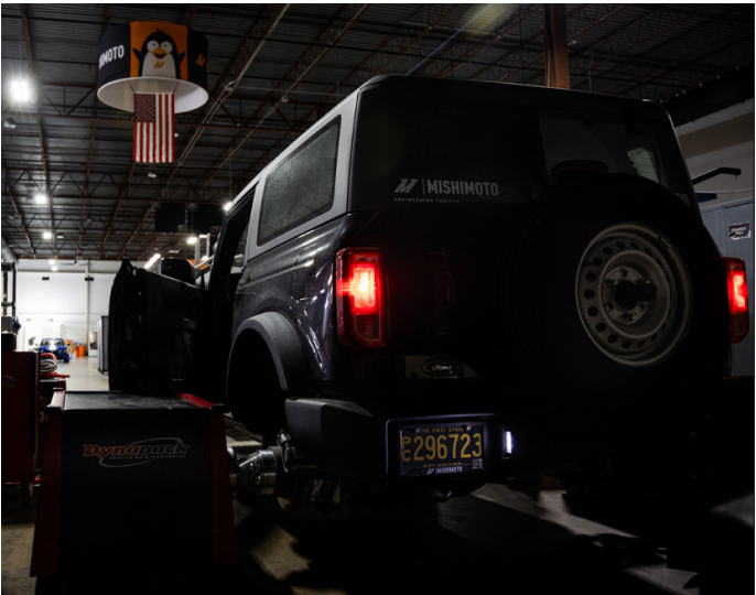
Figure 6: A Dynapack dynamometer was used for 2.3L testing.
