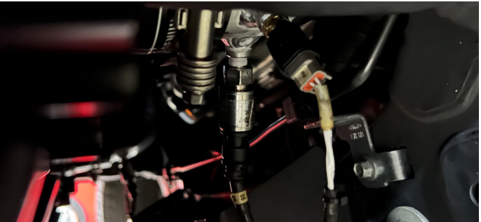
Figure 5: Pressure and temperature sensors installed in the cold-side intercooler piping.
