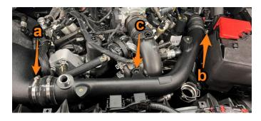
**8.** Using a 7mm socket, loosen the clamp on the passenger-side turbo.
