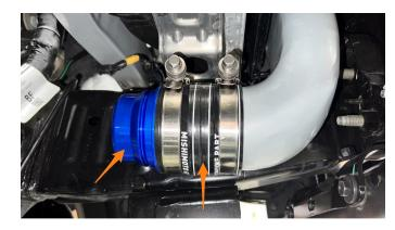
**20.** Install boot 7 onto the bottom of cold-side pipe 1 and hot-side pipe 3 with the smaller diameter inward. Push the boots all the way on as shown and slide 2x 92mm clamps on each pipe.
