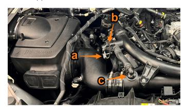
3. Using an 8mm socket, remove the three bolts securing the hot-side intercooler pipe to the air intake (a). Using a 7mm socket, loosen the hose clamp (b). Release the quick disconnect clip (c) and lift the passenger-side hot-side intercooler piping assembly out of the yehicle.
