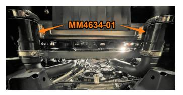
24. Using a 10mm socket and wrench, fasten the passenger-side intercooler pipe to the bracket with the provided 6mm bolt and nut. Install the longer straight section of boot 5 onto the pipe and slide 2x92mm clamps over the boot.
