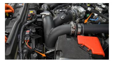
**33.** Install the assembly from steps 28/29 on the passenger-side of the engine, being sure to get the boot onto the turbo outlet and the other end of the pipe into the other side of the "Y" from the previous step.
