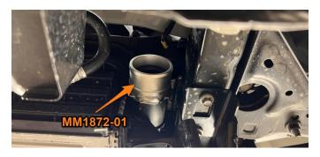
**18.** Swap the quick disconnect adapters on the Mishimoto stock-location intercooler for the silicone boot adapters. **Skip to step 20.**
