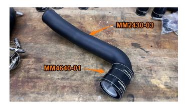
21. From the bottom of the vehicle, install cold-side pipe 1 on the passenger side and hot-side pipe 3 on the driver side. Reattach the ground strap from step 11. \*If using a stock intercooler or Mishimoto stock-location intercooler, proceed to step 22. If using a Mishimoto high-mount intercooler, skip to step 23.
