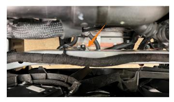
**12.** Using a 15mm socket, loosen the 2 rear bolts and completely remove the rest of the bolts. Remove the front skid plate/splash guard. Both the plastic splash guard and metal skid plate are shown on the top right. (Image on top right)
