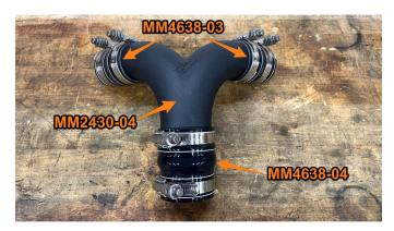
**31.** Install the assembly from step 27 on the driver-side of the engine, being sure to get the peg into the rubber grommet on the intake pipe and the boot onto the turbo outlet. The peg can slide in its slot to accommodate proper alignment.
