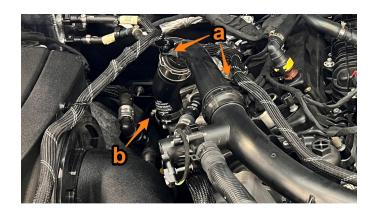
2. Unplug the recirculation valve connector (a) and remove the two wire clips (b). Disconnect the recirculation hose quick disconnect fitting from the air intake (c). Using an E5 Torx or 4mm socket, remove the 3 stud bolts and remove the valve from the stock intercooler pipe.
