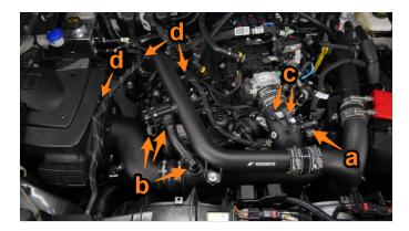
**38.** Loop one zip tie around the Mishimoto intercooler pipe on the driver-side. Loop another zip tie through the first one and around the vacuum hose. Pull tight and trim the ends. Repeat this process for the other vacuum hose.
