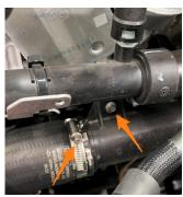
11. Using an 8mm socket, remove the bolt holding the ground strap and tuck the strap on top of the cross member.
