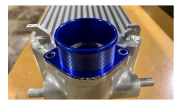
19. Remove the blue quick disconnect adapter and boot from the Mishimoto high-mount intercooler. Skip to step 21.
